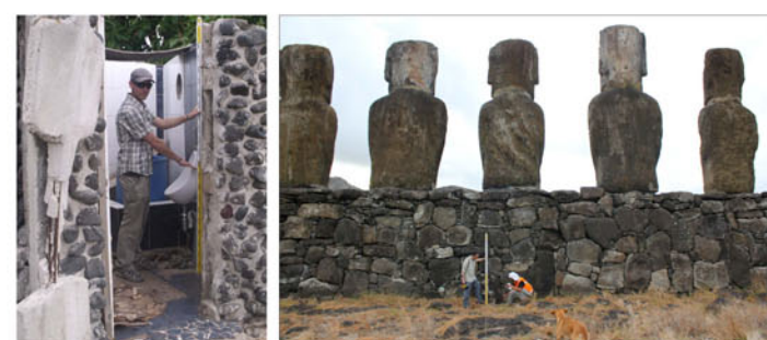
Figure 7. Tongariki, Rapa Nui: (a) flooded house; (b) eyewitness indicates inundation limit at the ahu with the moai statues.
